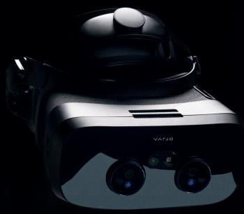
LiDAR and stereo RGB video pass-through deliver seamless merging of real and virtual for perfect occlusions and full 3D world reconstruction.
